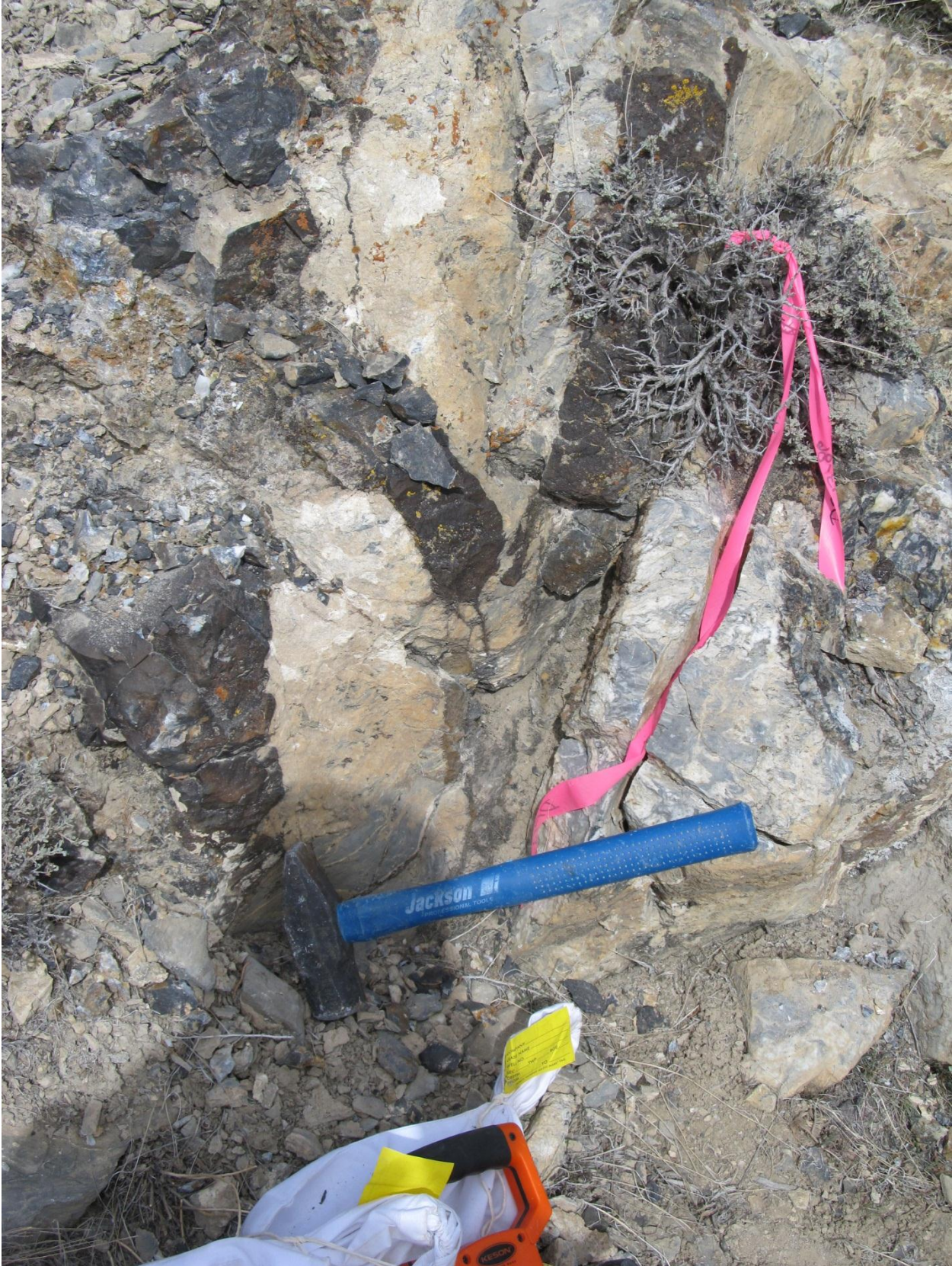
Figure 3. Black Jasperoid along Northeast Fractures, North target Area. Sample DP13-96—1.24 g/t gold, and 7.3 g/t silver.
